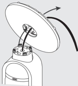
Attach the base to the fan bottom.
